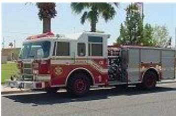
1997 Pierce Saber Pumper, Shop 420, 1500 GPM Waterous Pump, 750 Gallon Tank
